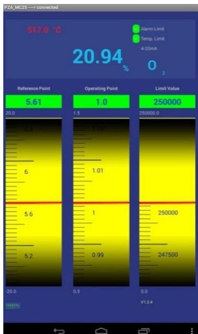
The display is now much more brightly lit. **ATTENTION!** The Reference Point, Operating Point, and Limit Value can now be adjusted. Changing the 'Reference Point' and 'Operating Point' affects the reading currently displayed and the reading output. We recommend that you read the 'Input explained' section before making the adjustments.
