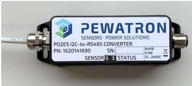
Figure 1 Modbus adapter box prototype. On the right-hand side with RS485 Modbus M12 TE Socket; on the left-hand side with attached strain relief and sensor cable.
