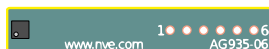
AG035-06: DFN6 connection board for -10E suffix sensors. (1.57" x 0.25" / 40 mm x 6 mm; actual size).
