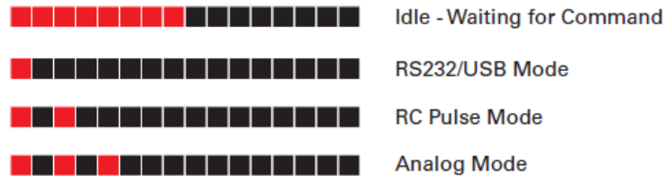
FIGURE 10. Normal Operation Flashing Patterns
