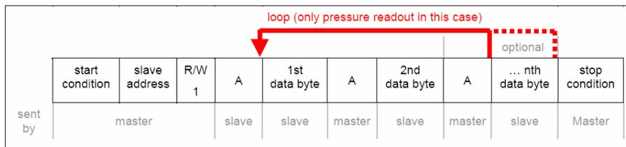
Fig. 2: Read operation - data request I<sup>2</sup>C
